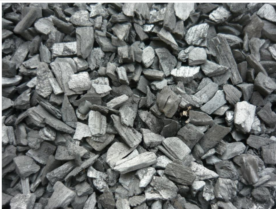
Picture 1: Terra-Preta biochar product recovered from wood chips and processed by “3R” high temperature pyrolysis process.
