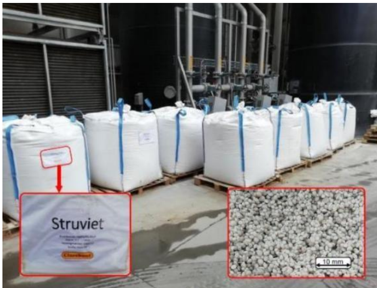
Figure 1. Big bags of Nuresys' struvite. In the right you can also see an example of the size of the microgranules.
