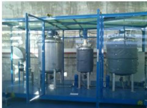
Figure 1. VALUVOIL two-phase anaerobic digestion plant
