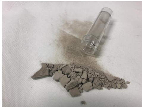
Figure 1. REVAWASTE Process Struvite
