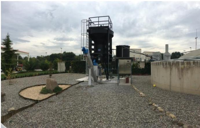
PHORWater crystallization reactor.
